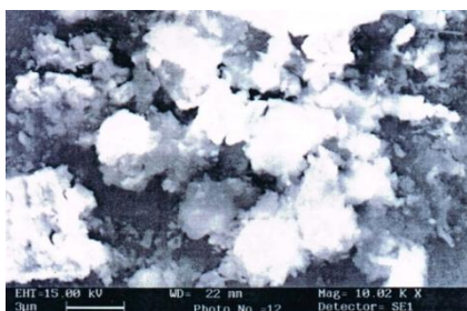
Fig. 1.4 SEM image of Pani/CdS thin film on to glass substrate.
